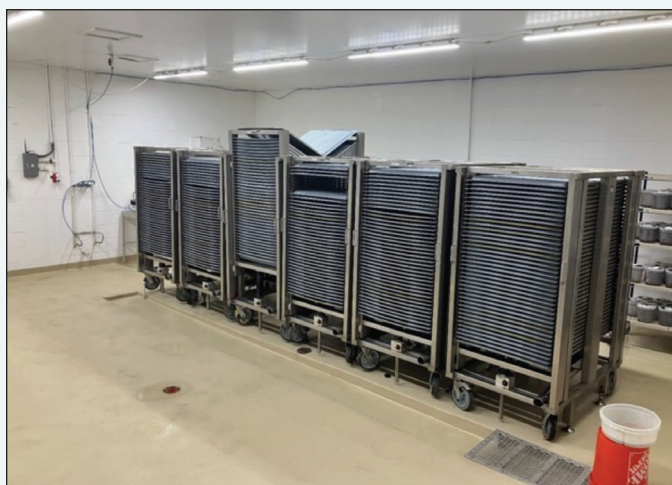
Fig. 1. Larval rearing racks for mass production of mosquitoes.
