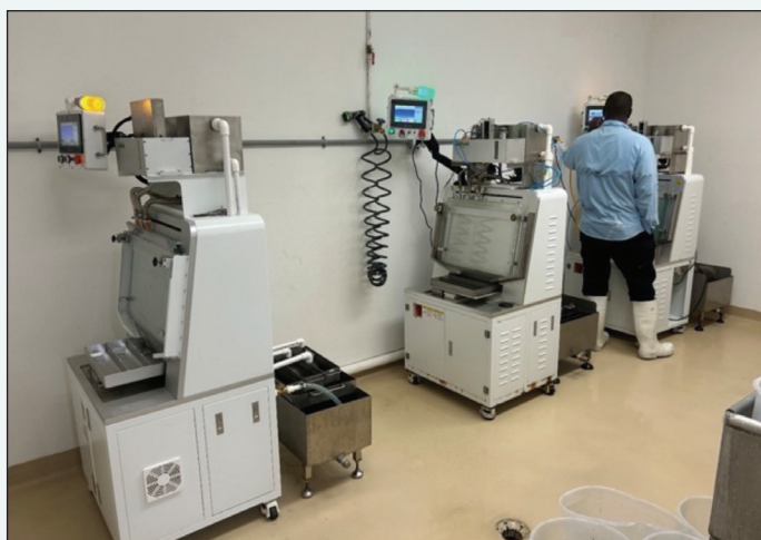
Fig. 2. Automated separation units for separating male and female mosquito pupae.
