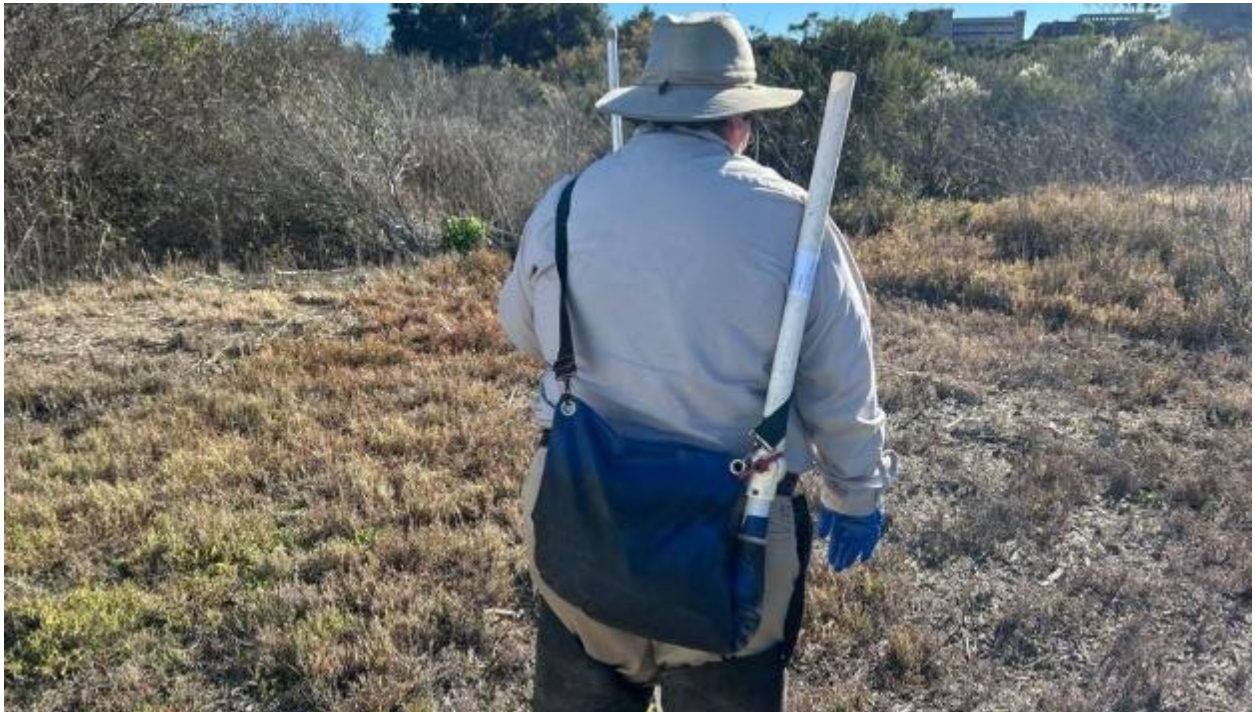
Photograph 10. View of horn seeder equipment carried by District field technicians to deploy granules. The horn seeder includes a heavy duty vinyl bag that holds granules, and a PVC pipe that disperses them. (December 10, 2025).
